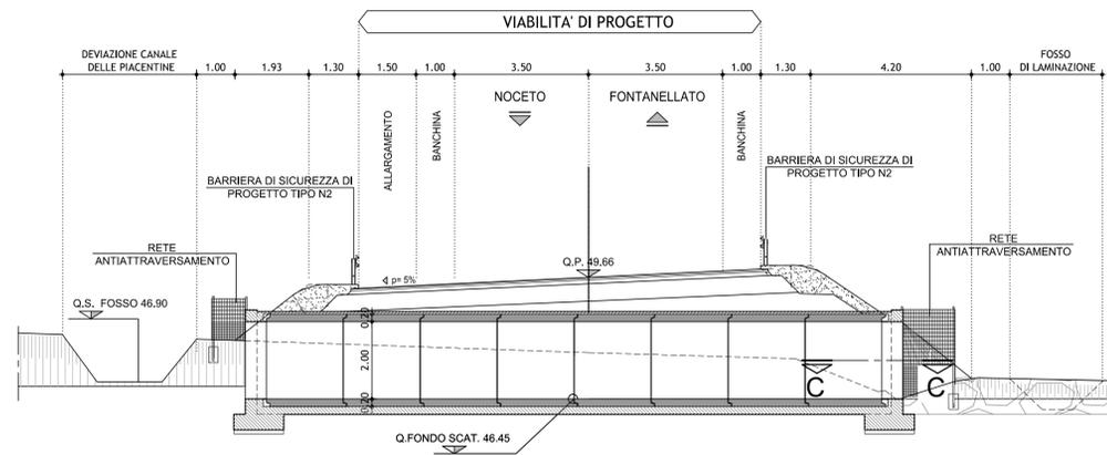
PIANTA SCATOLARE 200x200 IDRAULICO-FAUNISTICO
